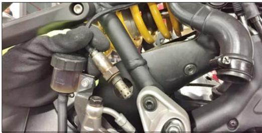
**ENG** Unscrew and remove the lambda probe
