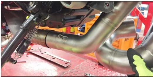
**ENG** Starting by placing the Termignoni collector (1) in the orizontal head pipe.
