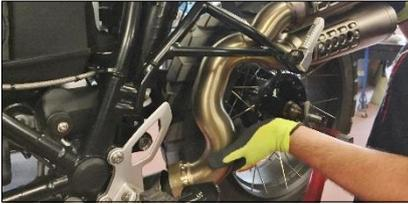
**ENG** Unscrew the screw of the silencer support bracket, keeping it for mounting the Termignoni kit, and remove original exhaust and the small metal clamp
