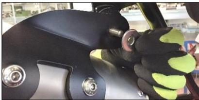
**ENG** Screw the silencer to the frame using the original screw and washer without tightening
